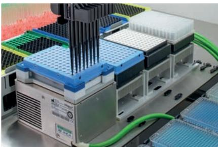
**Heating and cooling devices** – for sensitive reagents and incubation steps\*\*
