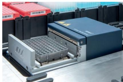
**Thermal cyclers** – integrated PCR for complete workflow automation\*\*\*
